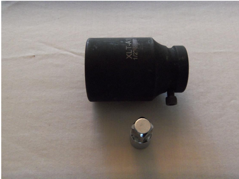
Above is the 6-point Grain Coupler mainly used on Timpte brand trailers.
